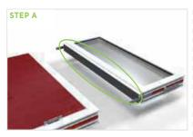
Inspect the coupler of the toplight that is factory fixed to the toplight frame. Confirm the grey intumescent 1mm thick pad that is applied to the coupler face where it will join to the doorset frame is not damaged. If it is damaged – do not proceed and contact Door-Stop for replacement.
