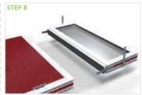
Screw (minimum size  $4.3 \times 40$ mm) fix  $1 \times 10^{-2}$  VEKA steel frame strap to both vertical parts of the toplight frame. They should be positioned approximately centrally along the length.
